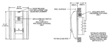
FLUSH INSTALALTION USING P-024900 STEEL BOX
